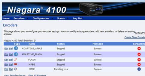
This web-based user interface allows you to browse to any Niagara 4100 on a LAN or WAN and manage the following system configurations:
