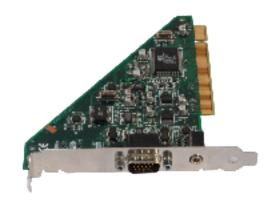
With on-board analog stereo audio inputs, the Osprey 210 is perfect for low-cost systems needing one video input and one unbalanced audio input. Monitor audio capture with enhanced sound capture at lower bit rates at an attractive price.
