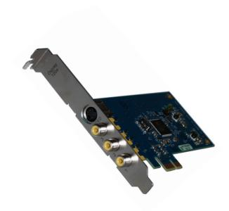
The Osprey 100e video capture card offers high-quality video capture at a reasonable cost. This low-profile, single-channel card has switchable inputs and is compatible with DirectShow applications.
